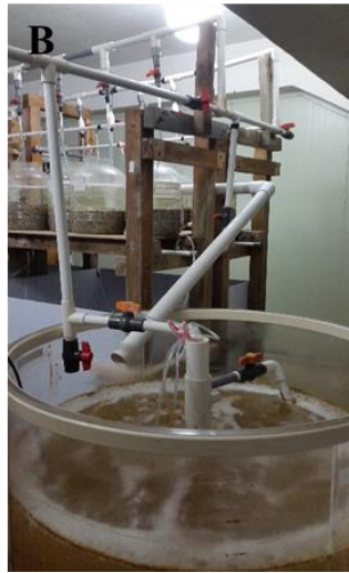
Fig. 5. The second experiment set-up. (A) arrangement of rearing bottles in the experiment room, (B) acrylic tank for biofloc preparation, and (C) outlet connected with \varnothing 50 mm PVC pipe lines.
