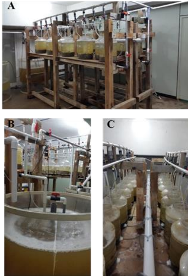
Fig. 4. The first experiment set-up. (A) arrangement of rearing bottles and an acrylic tank for biofloc preparation in the experiment room, (B) biofloc tank, and (C) PVC pipe line ( \varnothing 50 mm) with holes for adjusting water level by connecting with drainage outlets.
