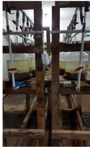
Fig. 5. The second experiment set-up. (A) arrangement of rearing bottles in the experiment room, (B) acrylic tank for biofloc preparation, and (C) outlet connected with \varnothing 50 mm PVC pipe lines.
