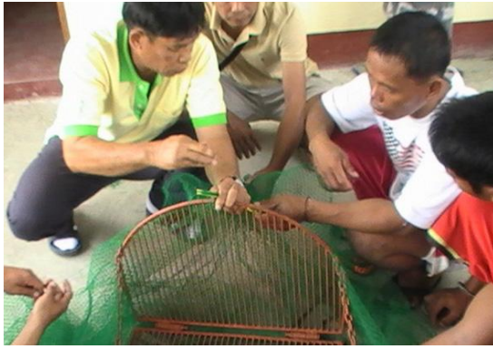
Practice on the installation of Juvenile and Trash Fish Excluder Device
